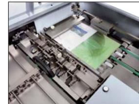
The jog guides are adjusted automatically according to the sheet size input on the SPF-30S. The gathered sheets are accumulated, jogged, registered and transported at a right angle to the scoring section.
