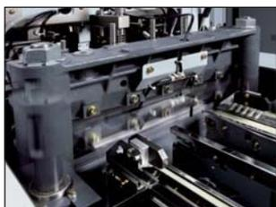
The servo-motor controlled feed mechanism provides for accurate booklet registration and fore-edge trimming. The guide is automatically adjusted according to the sheet size input on the touchscreen on the SPF-30S.
