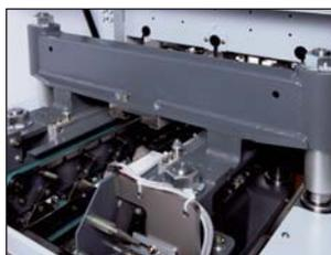
The top and bottom of the booklet are trimmed accurately, and trimming waste is smoothly extracted from the trim box to a movable chute with a powerful air blower. An optional center knife device can be fitted for two-up booklet production.
