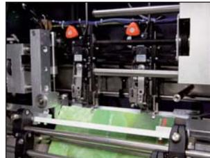
Booklets up to 10 mm thick (50 sheets of normal 80 gsm paper) can be stitched. The folded sets are jogged from the head and foot, then centered on the saddle by the centering mechanism before the heavy-duty stitching heads fire to
