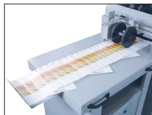
According to a preset number input on the touchscreen, a booklet is skewed to identify and separate the end of a series.
