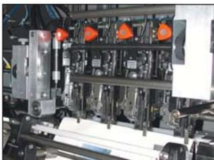
Standard stitcher head (#23 to #25 - thickness: 0.6 mm to 0.5 mm) and optional stitcher head (#25 to #27 - thickness: 0.5 mm to 0.4 mm) are available. Additional stitcher heads are available for up to 4 stitches per booklet with mounting block B-30S.
