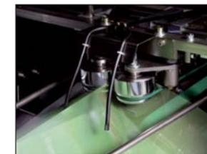
The scored sheets are folded reliably along the score line by a continuous series of forming rollers. The pressing rollers insure a sharp, tight fold.
