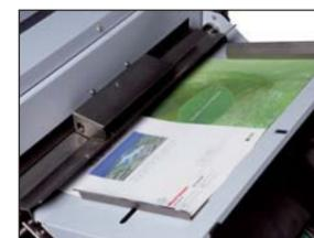
The ACF-30S is equipped with a hand feed unit for off-line bookletmaking and a misfeed tray for non-stop operation.
