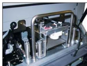
The HTS-TD is installed at fore-edge trimming section and checks the thickness of each booklet. In case of missing section or double sections, system stops for maximum quality control.
